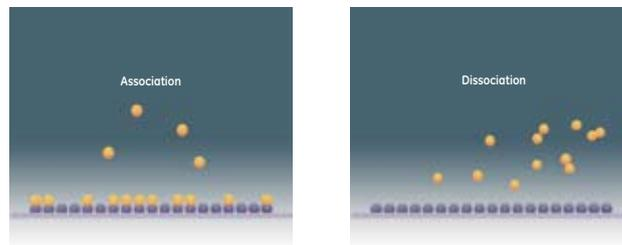
Intercalants in solution bind to molecules on sensor chip surface.
