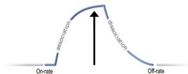
Real-time plots of binding response (the sensorgram) provides information on different kinetic profiles (*i.e.* on & off rates), affinities and protein concentration based on specific binding characteristics.
