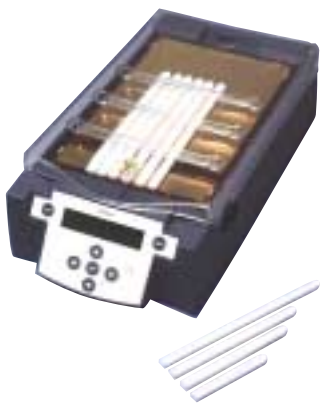
Fig 6. IPGphor Isoelectric Focusing System, a novel system for the IEF dimension of 2-D electrophoresis.
