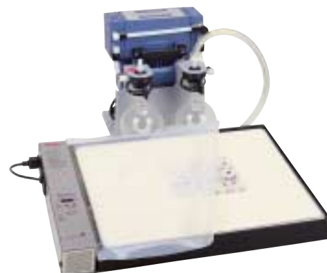
Fig 16. GD 2000 Vacuum Gel Dryer System dries acrylamide and agarose gels evenly.
