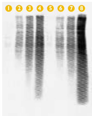
Fig 33. Comparison of results using Redivue Pro-Mix and the standard formulation Pro-Mix. Cell lysate products from in vitro cell labelling of NIH 3T3 mouse fibroblasts were separated by electrophoresis using an 8% polyacrylamide gel. Lanes 1–4, standard formulation Pro-Mix (0.125, 0.25, 0.5, and 1.0 mCi/ml, respectively). Lanes 5–8, Redivue Pro-Mix (0.125, 0.25, 0.5, and 1.0 mCi/ml, respectively).
