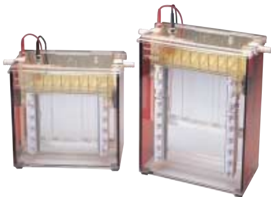
Fig 2. SE 600 vertical slab units run gels 8, 16 or 24 cm long.
