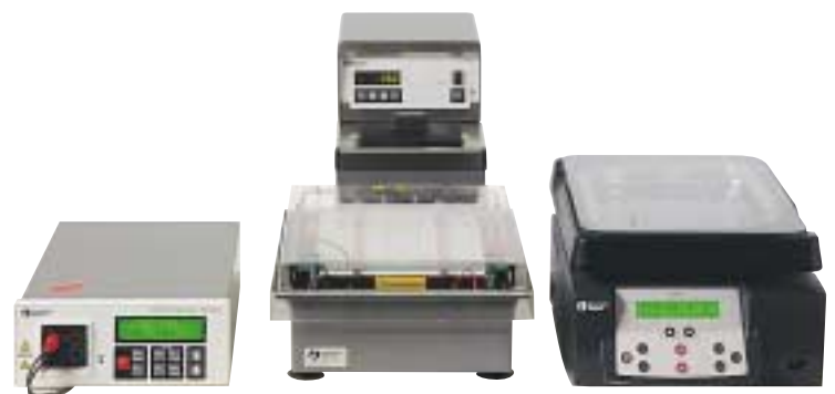
Fig 5. Complete Multiphor II Flatbed Electrophoresis System is designed for 1-D or 2-D electrophoresis.
