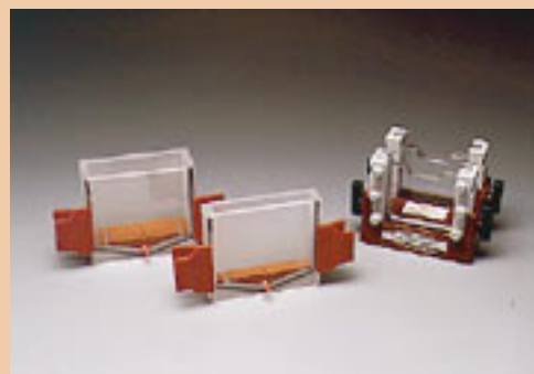
SE 275 Mighty Small Four-Gel Caster, SE 215 Mighty Small Multiple Gel Caster, and SE 245 Dual Gel Caster.
