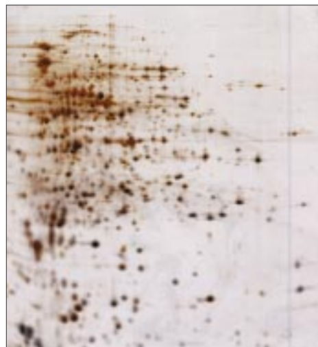
Fig 6. 2-D separation of an E. coli lysate. A 20-mg sample of E. coli lysate was separated on a 130 mm Immobiline DryStrip 3–10 L gel for the first dimension and a Hoefer SE 600 for the second dimension. First dimension separation was run for a total of 2 h 18 min (30 min at 500 V, 30 min at 1 000 V and 78 min at 8 000 V).
