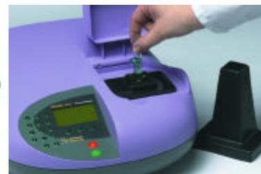
Fig 16. Test tube holder
