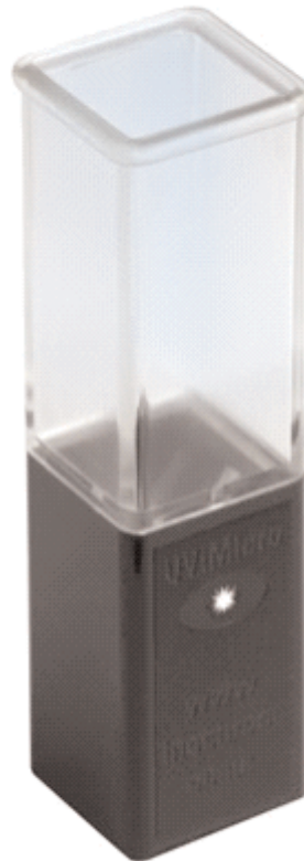
Fig 11. UViMicro disposable cell
