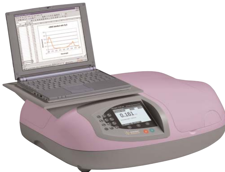
Fig 14. Ultrospec 2100 pro under PC control using SWIFT II
