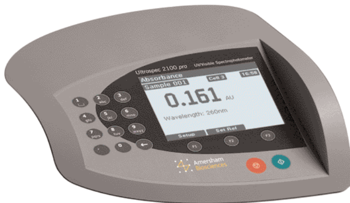
Fig 2. Ultrospec 2100 pro display and keypad
